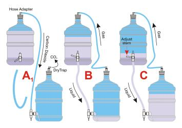
Optional, Better-Bottle PET Racking Adapters and SimpleFlo™ Valves makes it easy to rack under low oxygen, or oxygen-free, conditions, without siphons or pumps. Simply rotate the adapter, so its internal stem is above the sediment layer, open the valve, and let gravity do the rest. Connections are easily made using PET-lined tubing, which can be cleaned and sanitized in a flash. When it is time to bottle, a bottle-filling tube can be inserted neatly into the SimpleFlo™ Valve.
